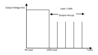
Additionally, if the I<sub>0</sub> is <210% but >150% for a prolong period of time (depending on the load), the Over Temperature Protection (OTP) will be activated due to high temperature on critical components. The power supply will then go into hiccup mode until the fault is removed; and, the input voltage is removed, then reapplied.
