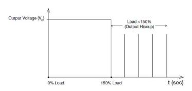
Additionally, if the  $I_0$  is <115% but >100% for a prolong period of time (depending on the load), the Over Temperature Protection (OTP) will be activated due to high temperature on critical components. The power supply will then go into hiccup mode until the fault is removed; and, the input voltage is removed, then reapplied.
