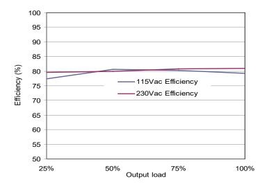
Fig.1 Efficiency versus output load
