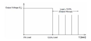
Additionally, if the  $I_0$  is <130% but >110% for a prolong period of time (depending on the load), the Over Temperature Protection (OTP) will be activated due to high temperature on critical components. The power supply will then go into hiccup mode until the fault is removed; and, the input voltage is removed, then reapplied.
