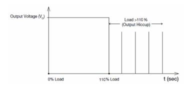
Additionally, if the  $I_0$  is <110% but >100% for a prolong period of time (depending on the load), the Over Temperature Protection (OTP) will be activated due to high temperature on critical components. The power supply will then go into hiccup mode until the fault is removed; and, the input voltage is removed, then reapplied.
