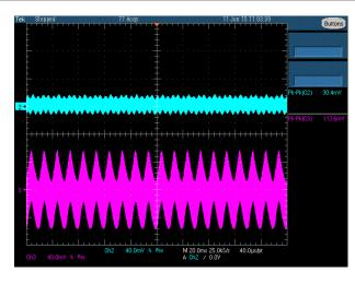
(a) 115V (measured value=112.0mV for 12V and 28.8mV for 5V) (b) 230V(measured value=113.6mV for 12V and 30.4mV for 5V)
