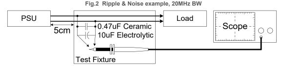
Fig. 3 Ripple & Noise measurement circuit
