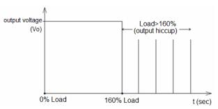
Additionally, if the 12 Volts' lout is >100%; but <160% for a prolonged period of time (depending on the load), the Over Temperature Protection (OTP) will be activated due to high temperature on critical components. The power supply will then go into latch mode.
