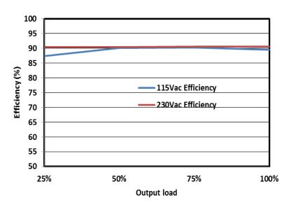
Fig.1 Efficiency versus output load
