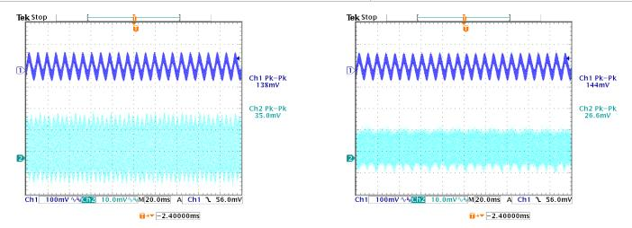
(a) 115V (measured value=138.0mV for 24V and 35.0mV for 5V) (b) 230V(measured value=144.0mV for 24V and 26.6mV for 5V)
