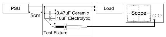
Fig. 3 Ripple & Noise measurement circuit
