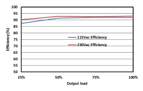
Fig.1 Efficiency versus output load
