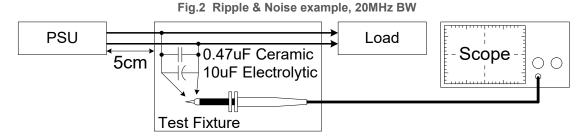
Fig. 3 Ripple & Noise measurement circuit
