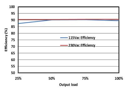
Fig.1 Efficiency versus output load
