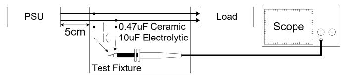
Fig. 3 Ripple & Noise measurement circuit
