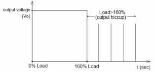
Additionally, if the 18 Volts' lout is >100%; but <160% for a prolonged period of time (depending on the load), the Over Temperature Protection (OTP) will be activated due to high temperature on critical components. The power supply will then go into latch mode.
