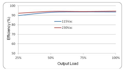
Fig.1 Efficiency versus output load
