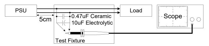
Fig. 3 Ripple & Noise measurement circuit
