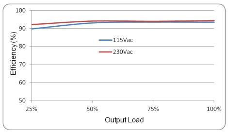
Fig.1 Efficiency versus output load
