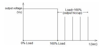
Additionally, if the 24 Volts' lout is >100%; but <160% for a prolonged period of time (depending on the load), the Over Temperature Protection (OTP) will be activated due to high temperature on critical components. The power supply will then go into latch mode.
