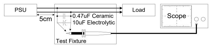
Fig. 3 Ripple & Noise measurement circuit
