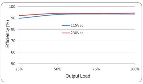
Fig.1 Efficiency versus output load
