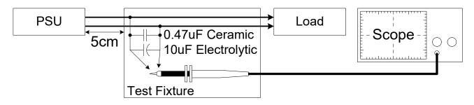
Fig. 3 Ripple & Noise measurement circuit
