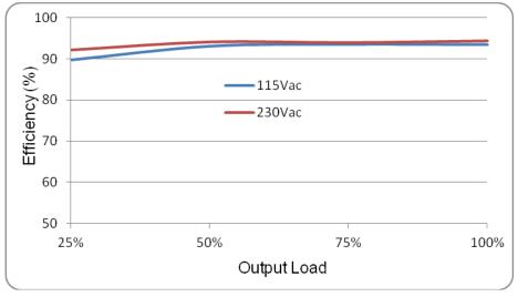
Fig.1 Efficiency versus output load
