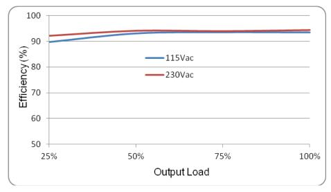
Fig.1 Efficiency versus output load
