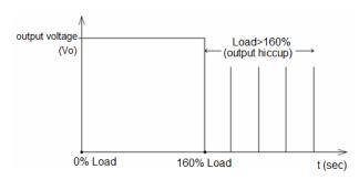
Additionally, if the 48 Volts' lout is >100%; but <160% for a prolonged period of time (depending on the load), the Over Temperature Protection (OTP) will be activated due to high temperature on critical components. The power supply will then go into latch mode.
