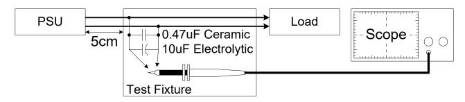
Fig. 3 Ripple & Noise measurement circuit
