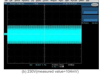
Fig.2 Ripple & Noise example, 20MHz BW
