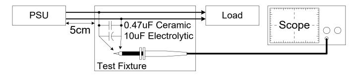
Fig.3 Ripple & Noise measurement circuit
