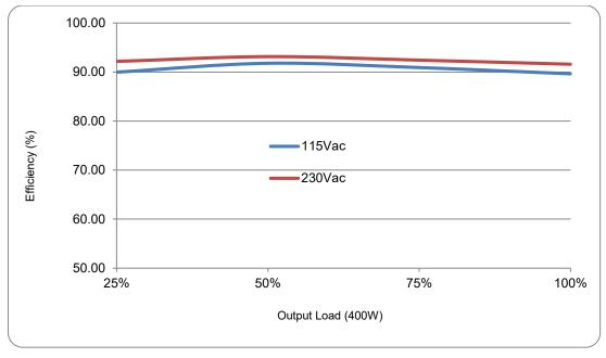
Fig.1 Efficiency versus output load
